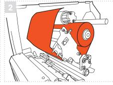
Route the ribbon through the ribbon sensor slot and up and over the print head. Tape the end of the ribbon to the blank cardboard core and wind the core up until the ribbon is tight and wrinkle free.
