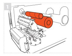
Lift the printer cover and print head mechanism (see supply instructions). Insert the ribbon onto the rear ribbon hub and the blank cardboard core onto the front ribbon hub.
