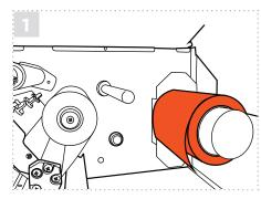
Lift the printer cover. Remove the green media cap from the media supply spindle and place the supply roll on the spindle. Replace the media cap so it sits snugly against the supply.
