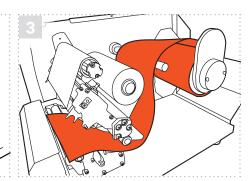
Route the supply over the silver media guide bar, under the spring loaded damper, between the green media alignment guides, and out through the mouth of the printer. Unlock the sliding alignment guide by pressing down and move it so it meets the edge of the supply. Close the print head mechanism (see ribbon instructions) and printer cover.
