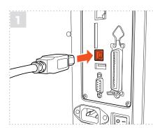
Connect the USB cable to the back of your printer and plug the other end into a USB port on your computer.
