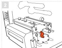
Push the print head release lever to open the print head mechanism.
