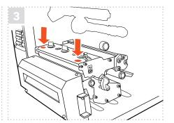
Close the print head mechanism by pressing down on both sides, making sure the latches are engaged properly. Then close the printer cover.
