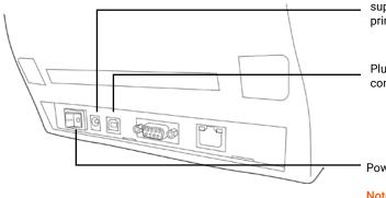
Connect power cable to power supply. Plug into the back of the printer, and wall outlet.
